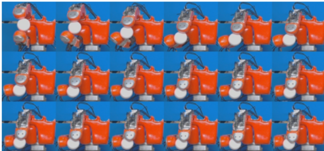
Fig. 6: Example of an in-hand manipulation for a sphere of diameter 30mm. Even though the initial grasping posture is out of the center of the fingertips ( x=-10\text{mm}, y=-10\text{mm} ) the handling was successful.
