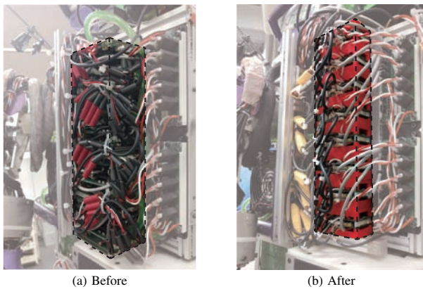
Fig. 18. Comparison backpack of JAXON1 before and after applying the tiny high-power motor driver.
