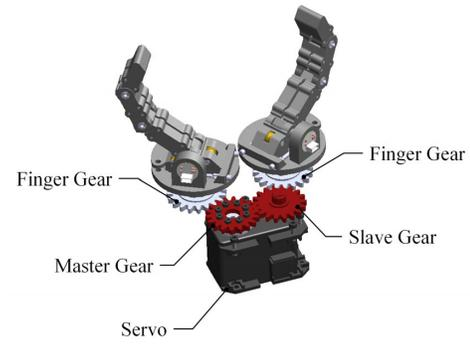
Fig. 2: Finger axial rotation powertrain contained in the palm.
