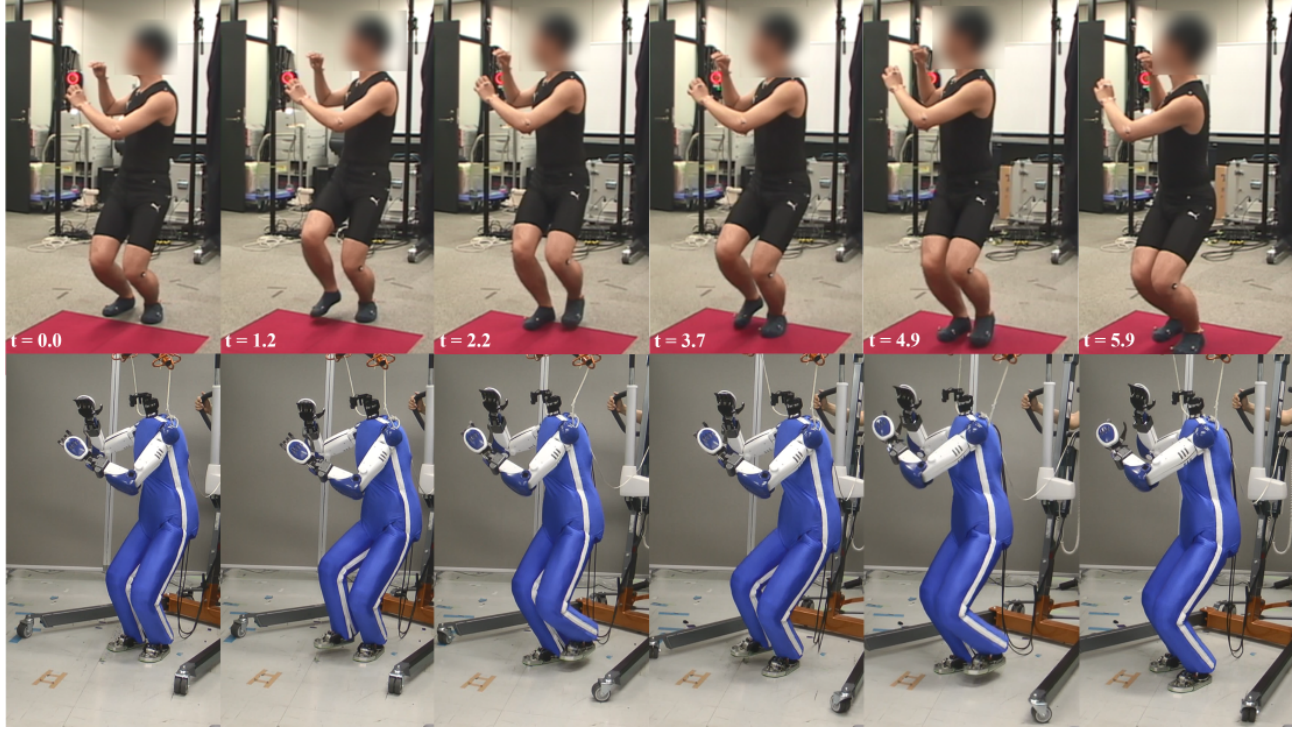
Fig. 6. Original human motion (top) and reproduced motion on HRP-4 (bottom). The motion includes four steps, and the timing of snapshots are the start and end, and each leg swinging.
