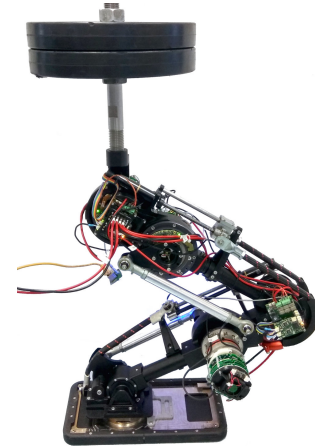
Fig. 1: Squatting eLeg in monoarticulated configuration with 20 kg load. In contrast, the robot weighs only 10.9 kg.
