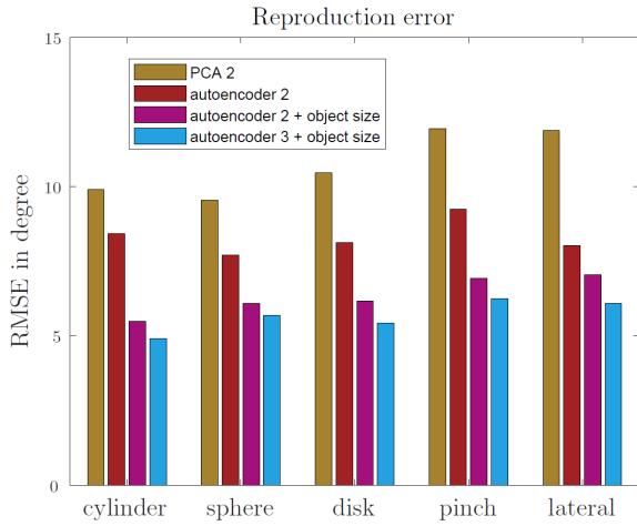
Fig. 4: Angular root mean squared error in the reproduction of human grasps for PCA and autoencoders with two variables in latent space with and without an additional parameter for object size compared to the presented autoencoder with three variables in latent space and object size
