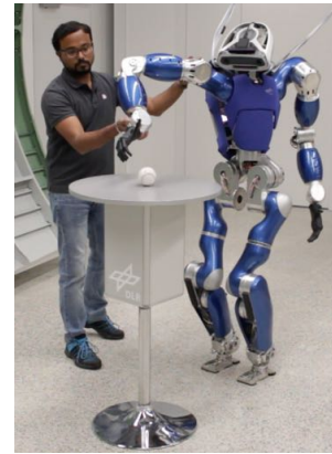
Fig. 1: Humanoid robot TORO [5] reaching to grasp a ball while actively balancing against the human perturbation.
