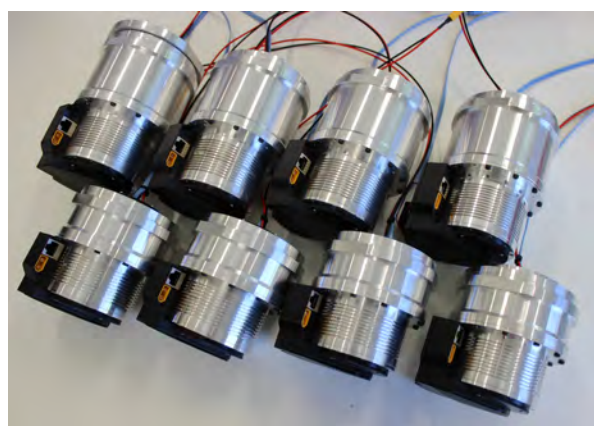
Fig. 3: Large and medium sized SAC units that power the arm joints of ARMAR-6, entirely developed and assembled at KIT.
