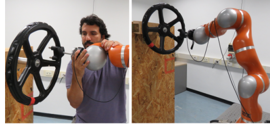
Fig. 1: Left : a human operator teaches a robot how to perform a valve-turning task. Right : a snapshot showing the valve-turning task reproduced by a KUKA LWR robot.
