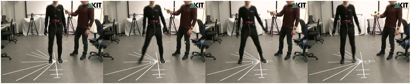
Fig. 5: Push-Recovery experiment in the motion capture lab. Temporal order of the images from left to right 0.2 s spacing.
