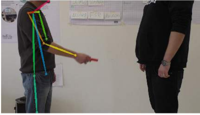
Fig. 3: Sample image of the video analysis with the RGB camera. The left person hands over an object with his right hand. The positions of the joints and limbs have been detected and highlighted with OpenPose.
