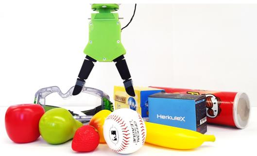
Fig. 17. Grasping Testing of the two-fingered robotic hand
