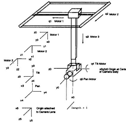
Figure 1: 5-DOF Hybrid Robot
