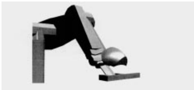
Fig. 16. The merged candidate volume V_C , embodying all task constraints, along with the swept robot model and the fixtured object.
