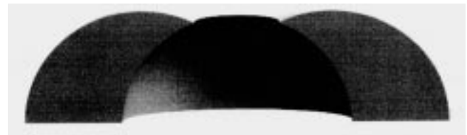
Fig. 14. Candidate volume for one linear feature, considering only field-of-view and resolution constraints. The figure has been cut away twice to show the inside, but the actual volume is symmetric about the two cutaway planes.
